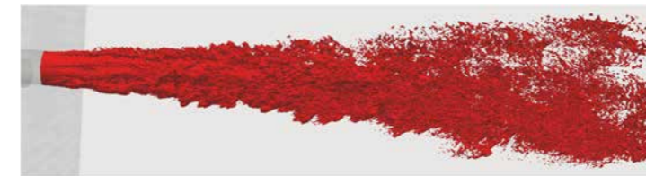
Figure 1: Representative quasi-stationary simulation snapshot visualized by isosurface of liquid volume fraction with value \alpha = 0.5 .
