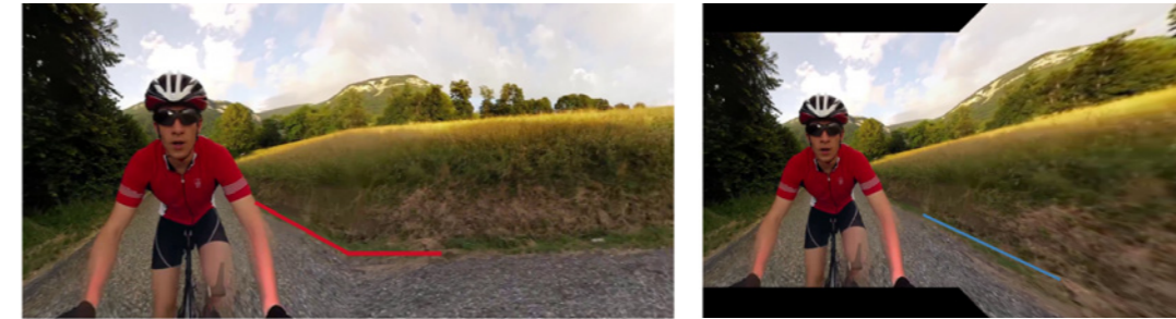
Figure 2: (a) Face A and B. Red: Geometric distortion at face boundary (b) Blue: Corrected geometric distortion.
